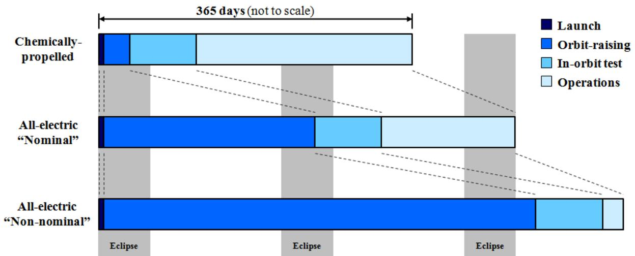
Fig 3: Typical mission phases including “non-nominal” all-electric GEO comsat
