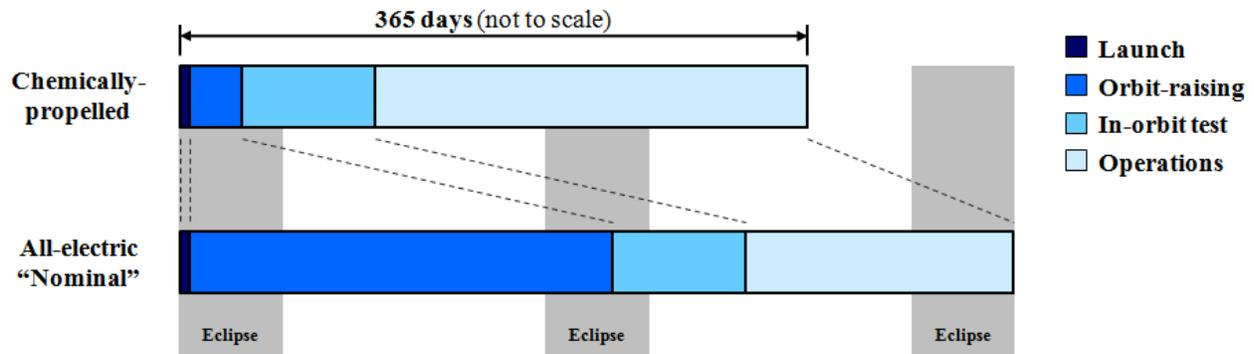
Fig 2: Typical mission phase durations for chemically-propelled and “nominal” all-electric GEO comsats
